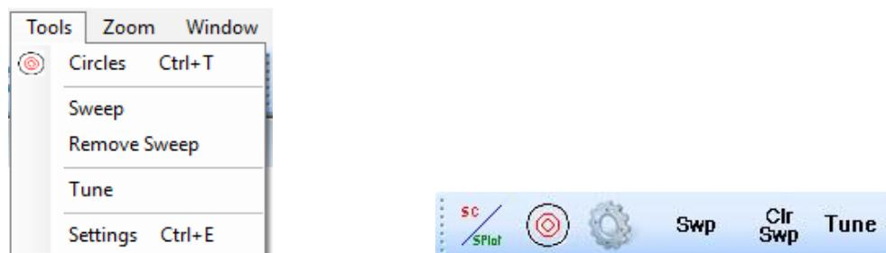
Before doing a sweep design a network starting from one datapoint. For datapoint sweep all datapoints must be input before starting a sweep.
